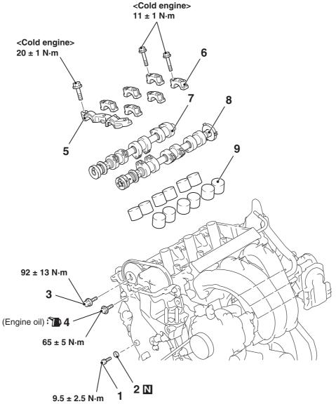
Apply engine oil to all moving parts before installation.
