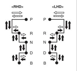
: Turn the ignition switch to the "ON" position, and operate the lever while depressing the brake pedal.
