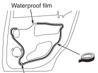
Inner panel water drain hole
