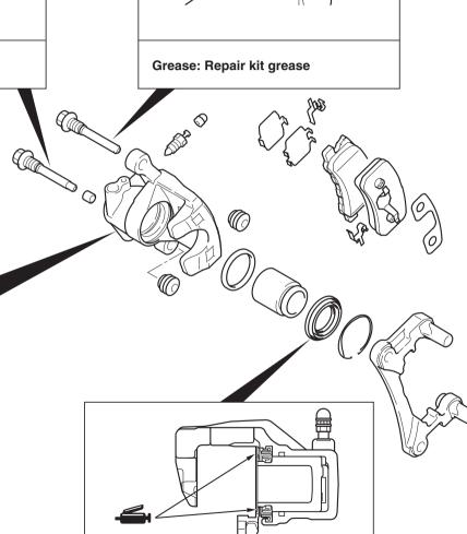
Grease: Repair kit grease
