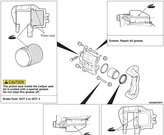
Grease: Repair kit grease
