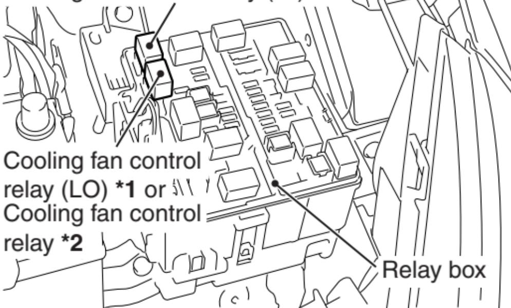
Cooling fan control relay (HI) \*1
