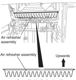
Assemble into the heater side cover in this direction.
