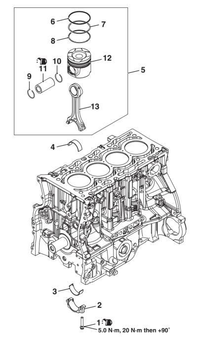
Apply engine oil to all moving parts before installation.
