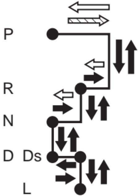
→ : Turn the ignition switch to the "ON" position, and operate the lever while depressing the brake pedal.
