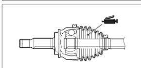
Grease: repair kit grease Amount used: 120 ± 10 g
