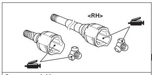
Grease: repair kit grease Amount used:
