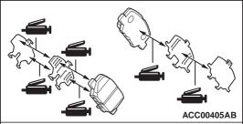
Grease: Repair kit grease, AS880N or equivalent
