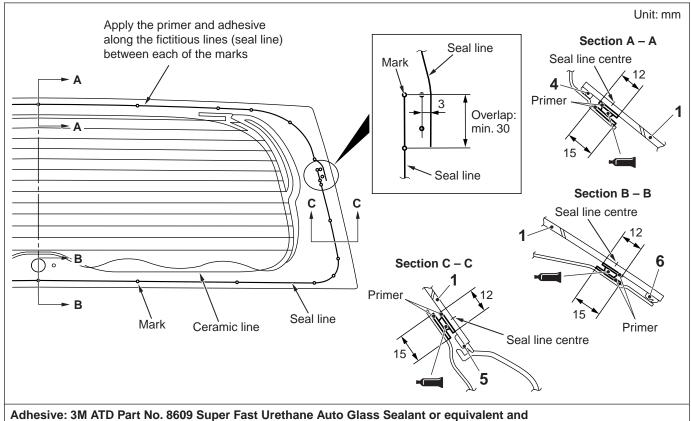
Adhesive: 3M ATD Part No. 8609 Super Fast Urethane Auto Glass Sealant or equivalent and 3M ATD Part No. 8608 Super Fast Urethane Primer or equivalent
