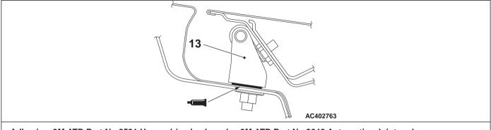
Adhesive: 3M ATD Part No.8531 Heavy drip check sealer, 3M ATD Part No.8646 Automotive Joint and Seam Sealer or equivalent
