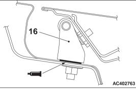
Adhesive: 3M ATD Part No.8531 Heavy drip check sealer, 3M ATD Part No.8646 Automotive Joint and Seam Sealer or equivalent
