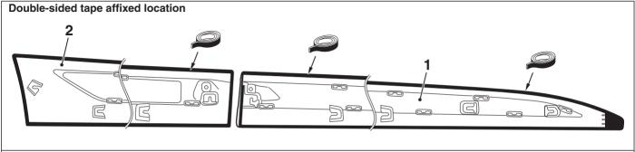
Double-sided tape : Generic products 4.0 mm width and 1.2 mm thickness
