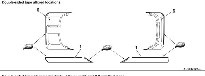
Double-sided tape: Generic products, 4.0 mm width and 0.8 mm thickness
