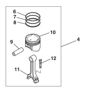
Apply engine oil to all moving parts before installation.
