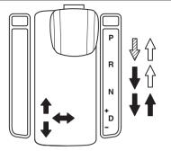
The selector lever moves when the brake pedal is depressed and the button is pushed in with the ignition key in any position other than the LOCK (OFF) position.
