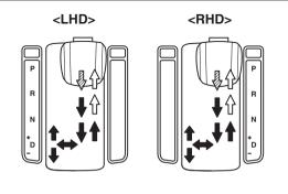
The selector lever moves when the brake pedal is depressed and the button is pushed in with the ignition switch at ON position.
