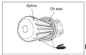
Grease: Multi purpose grease SAE J310, NLG1 NO.2 or equivalent (Spline: approx. 9 g, Oil seal lip: approx. 3 g)
