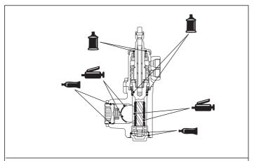
Grease: Repair kit grease
