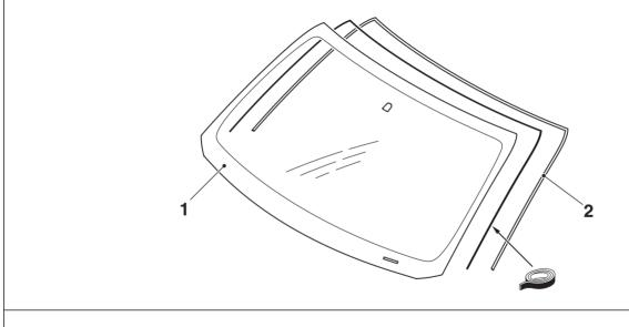
Adhesive tape: Double-sided tape: 6.0 mm width, 2,522 mm length and 0.15 mm thickness
