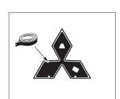
Adhesive tape: Double-sided tape, 0.8 mm thickness
