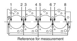
Protrusion measuring locations (with each piston at top dead centre)
