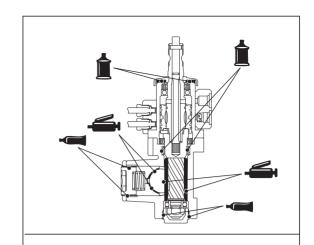
Grease: Repair kit grease
