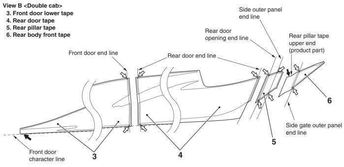
← : Align the tape end with the front door character line/rear pillar tape upper end (product part). <□ : Align the tape mating notch to front door/rear door/rear pillar/side gate end line
