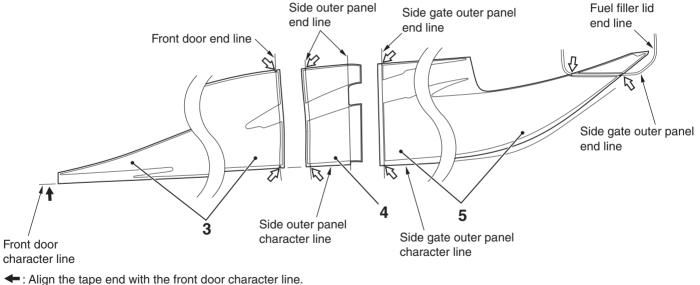
←: Align the tape mating notch to the front door/side outer panel/side gate outer panel/fuel filler lid end line.
