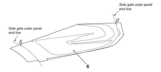
: Align the tape mating notch to the side gate outer panel end line.
